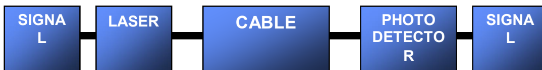
Fig. 1: Fiber optic transmission
