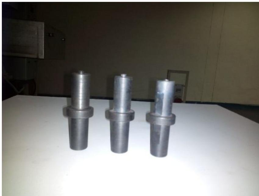
The specimen size of the copper plate that is used for processing 200 mm x 74 mm x 5 mm. One groove of 1mm width and 2 mm deep was made on the 99.99% pure Copper Plates using horizontal milling machine with a 1mm (width) saw cutter was cut in the middle of the specimen plate for processing. The tool Material used is H13 steel with shoulder diameter 15mm, threaded pin diameter 8 mm, pin length 2.5 mm with tool rotational speed 960 rpm, tool angle 2° and table traverse speed 25 m / min.
